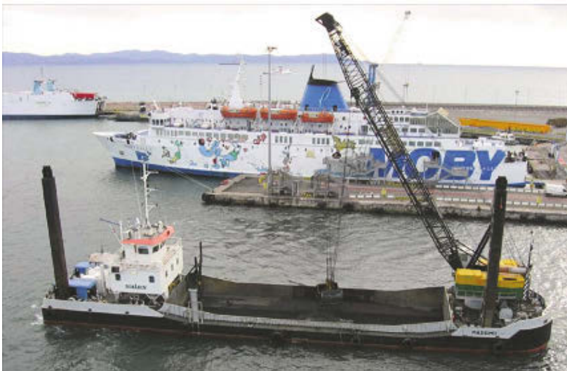
Figure 4 - Spilt-barge motor ship used for the removal of clods.
